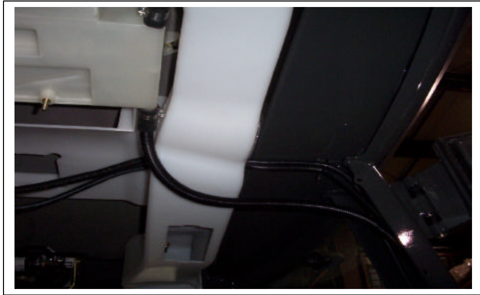
Left rear drain tube
